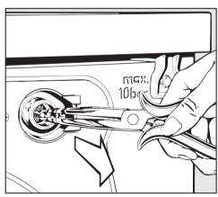
Using needle nose pliers, withdraw the plastic filter by pulling on the bar (see illustration). Rinse under water and return parts.
